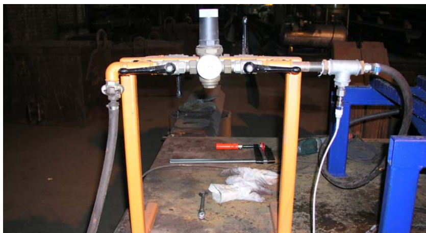
Figure 3: Pressure control system with manometer
