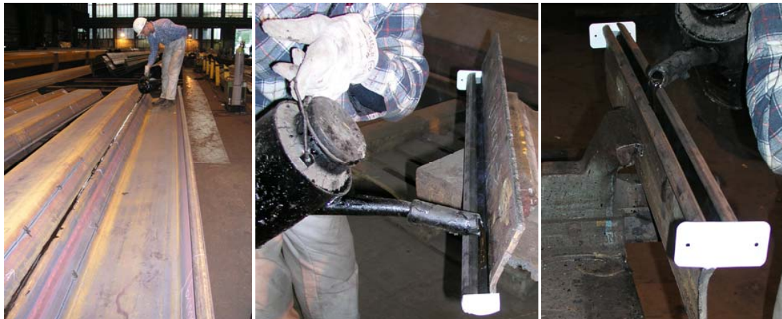
Figure 7: Application a) LARSEN Middle Interlock, b) LARSEN Site Threading Interlock, c) PZ Site Threading Interlock (“Ball and Socket”)
