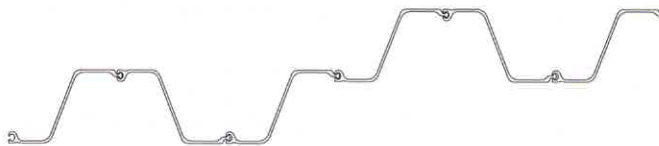
Layout to Shift the Line by the Depth of One Sheet
