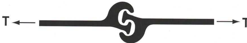
Tensile Diagram For Properly Interlocked PS Sections
