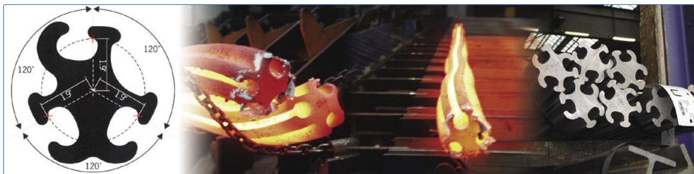
Figure 3. Pile Properties and Extrusion Process for the SWC 120 Pile.
